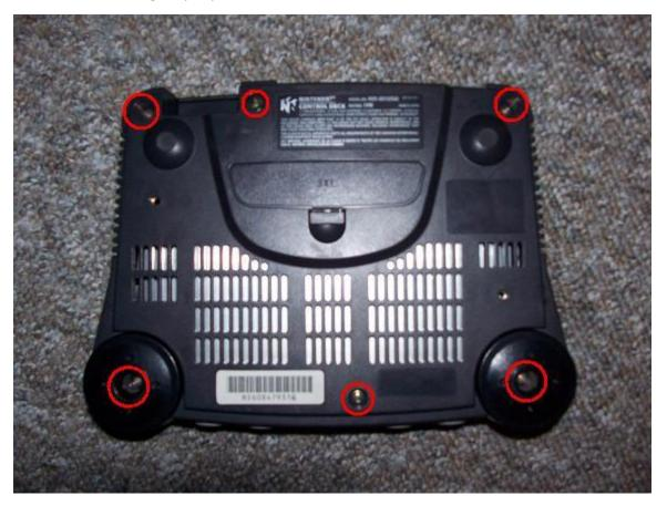
The screws are in the red circles. Remove them, and you should be able to separate the two halves. Oh, and don't panic when the front feet come off. It's supposed to happen.
